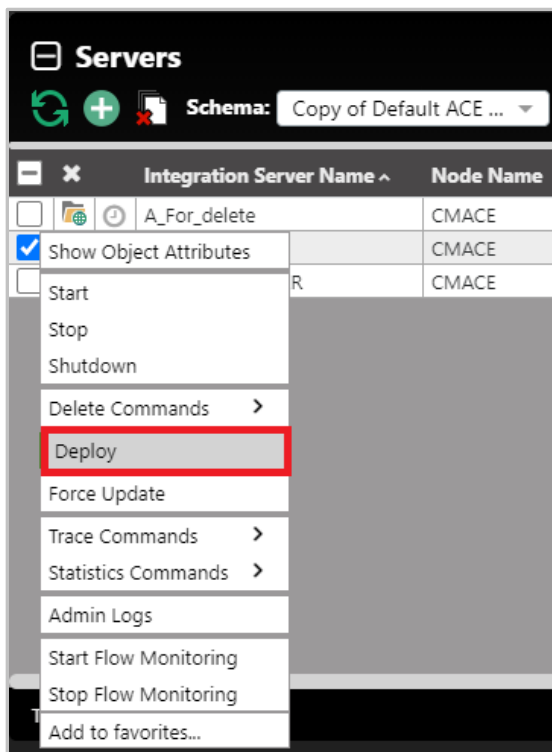
Figure 4.3.16.4-A. Select Integration Server > Deploy
